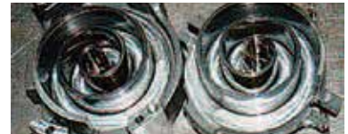
Sludge (carbide) deposits
